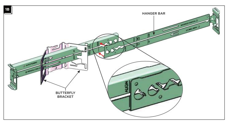
2 Invert and align the other hanger bar against the previously installed hanger bar using the "ALIGN" marking.
