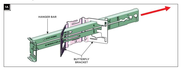
1 Slide the hanger bar into the butterfly brackets through one of the suitable locations.
